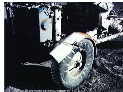
Fender Repair on Apollo 17
