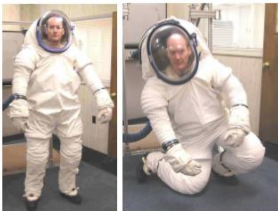
I-Suit with a modified DuPont Tyvek® cover garment in first order interface test
