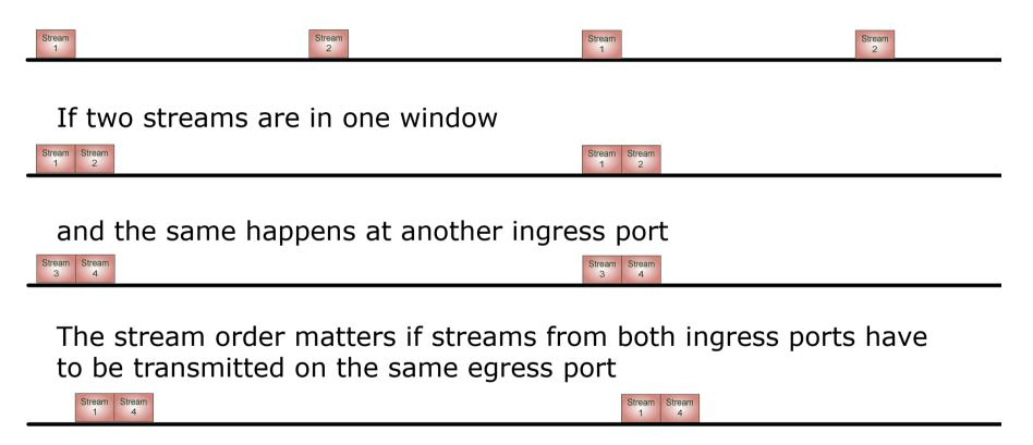
Even with one window per cycle it is necessary to have "small windows" within the big window
