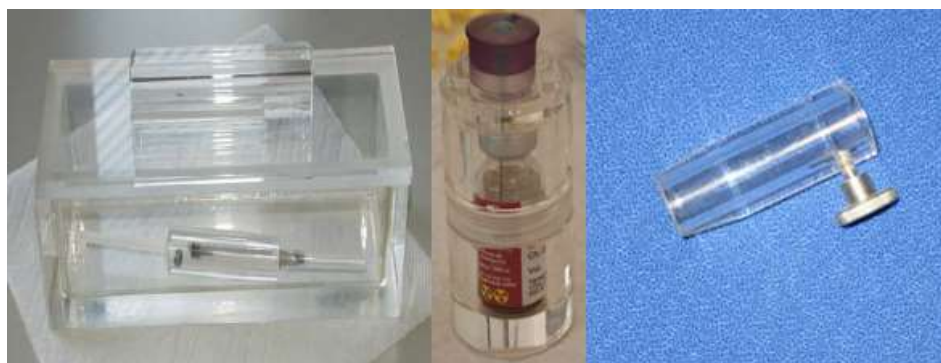
FIG. 34. Plexy shielding for syringes and vials (courtesy of Farahati)
