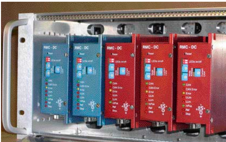
Test chassis with multiple units of the ESO-developed CAN-bus DC motor drive module.
