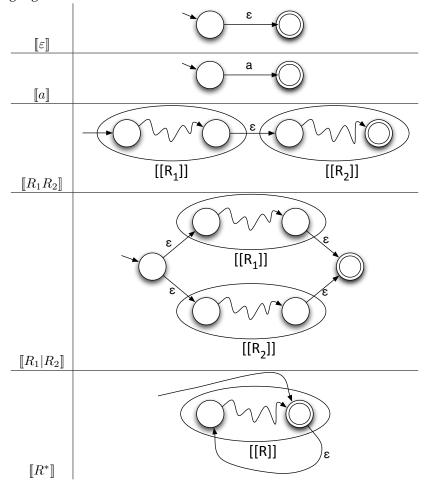
By working bottom up, we can use these translations to construct an NFA for any regular expression. For example, the odd number regular expression above,  $(0|1)^*1$ , translates to the following NFA, which clearly accepts the same strings. (The states in this diagram are labeled with names A–G for later use).
