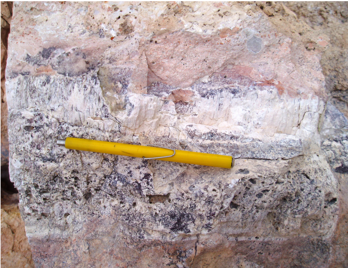
Figure 17. Alunitic vein in massive quartz-alunitic sample from Blawn Mountain.
