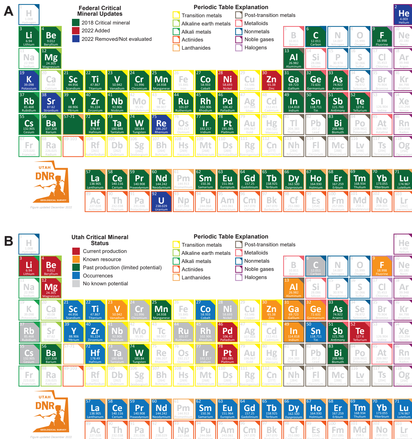
Figure 1. (A) Periodic table showing changes between the 2018 and 2022 federal critical minerals identified by the U.S. Geological Survey, and (B) periodic table highlighting critical minerals found in Utah, highlighted according to their current resource status.
