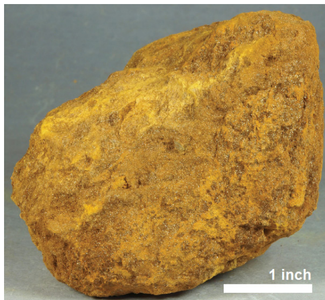
Figure 21. High-grade Ge-Ga plumbojarosite ore from the Apex mine. Photo from Wenrich and Verbeek (2014), reproduced with the permission of Utah Geological Association.
