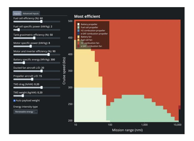
The StratiFly tool allows users to visualize how shifting technology assumptions (left) impact the most efficient propulsion system for each combination of cruise speed and mission range (right). Credit: *Progress in Aerospace Sciences* (2024). DOI: 10.1016/j.paerosci.2024.101051
