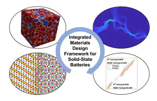
Diagram illustrating the integrated computational framework used to design materials for solid-state batteries. The framework incorporates atomistic simulations of local bulk and interfacial properties, representative multi-phase polycrystalline microstructures, effective property calculations and a machinelearning analysis to correlate microstructure features with effective properties. Credit: Lawrence Livermore National Laboratory
