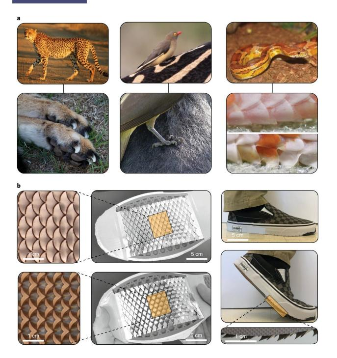
a, Inspiration from friction-enhancing strategies in animals: cheetah with semiretractable claws (left), oxpecker with sharp claws in opposing directions (middle) and snake with scales that are oriented to increase friction (right). b, Kirigami for friction modulation in footwear. Steel kirigami surfaces were attached to the shoe soles (middle). The undeformed (top) and deformed (bottom) configurations of the kirigami shoe grip are illustrated. The spikes are
