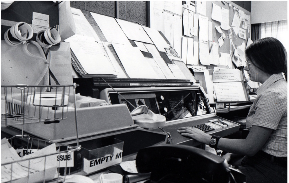
Paper tape spools being used for newspaper typesetting, circa 1976. Source: Gordon Haff.
