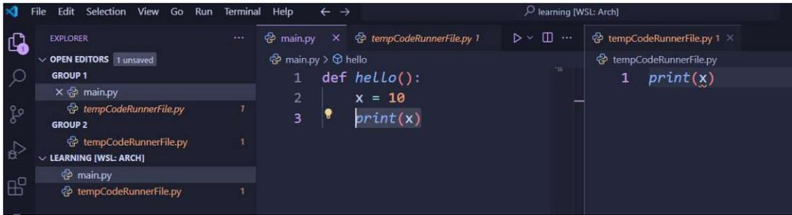
Figure 2.1: **Code Runner example** - Original code file (`main.py`) containing the selected code line 3 (`print(x)`) alongside the temporary file `tempCodeRunnerFile.py` which was automatically generated by Code Runner. The `tempCodeRunnerFile.py` demonstrates that only the selected code was copied into a temporary file for execution, without resolving dependencies within the selected code.
