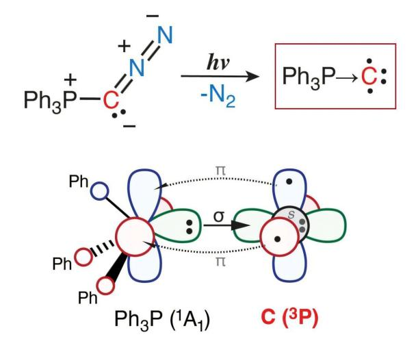
Synthesis of monosubstituted  $Ph_3P \rightarrow C$  by light-triggered dinitrogen elimination (top) and theoretical description of the bonding (bottom) showing that the carbon exists in its atomic triplet ground state. Credit: Max Planck Society
