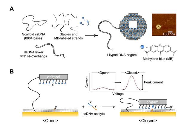
Lily pad sensors can be used for the electrochemical detection of biological analytes, here a DNA single strand. Credit: Byoung-jin Jeon et al
