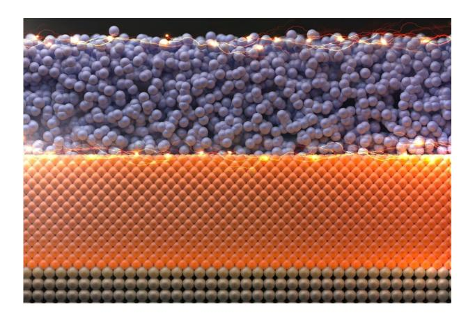
A film a few atoms thick of non-crystalline niobium phosphide conducts better through the surface to make the material, as a whole, a better conductor. Credit: Il-Kwon Oh / Asir Khan
