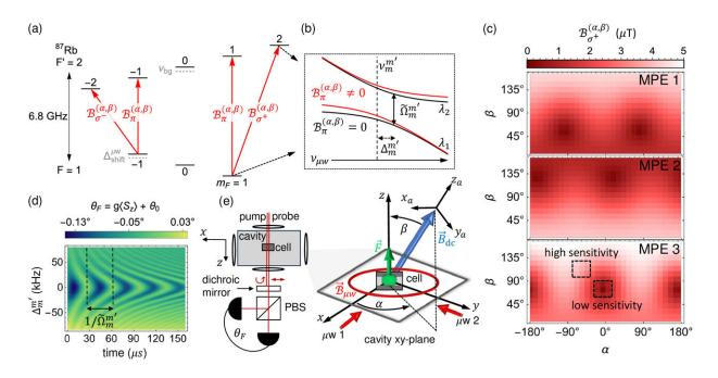
Vector magnetometry using Rabi oscillation frequencies referenced to multiple microwave polarization ellipses (MPEs). Credit: *Optica* (2024). DOI: 10.1364/OPTICA.542502
