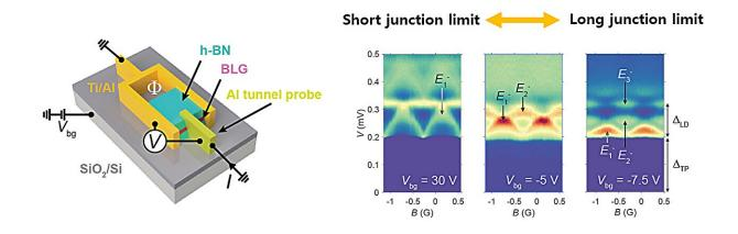
A schematic of a bilayer graphene Josephson junction device with a tunneling electrode. Credit: POSTECH
