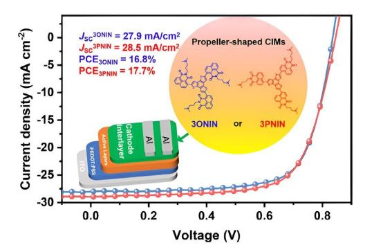
Due to the difference in planarity of the two isomers 3ONIN and 3PNIN, 3PNIN based OSCs show a higher power conversion efficiency relative to 3ONIN based devices. Credit: Minghua Huang, Ocean University of China
