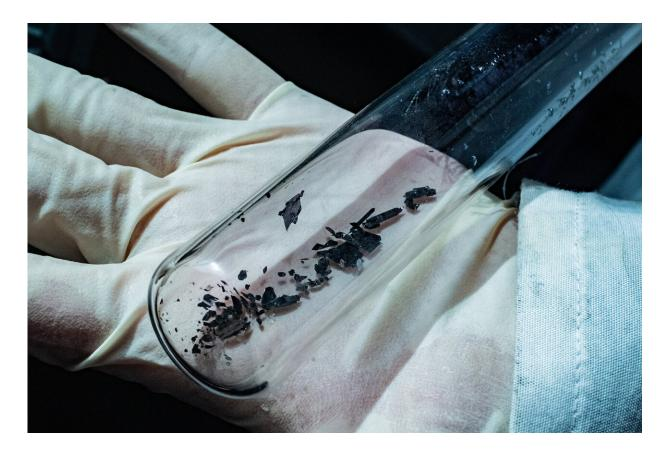
Graduate student Lebing Chen displays chromium triiodide crystals he made in a Rice University laboratory. Stacked layers of atomically thin 2D chromium triiodide have unusual electronic and magnetic properties that could prove useful for technologies that encode information in the spins of electrons. Credit: Jeff Fitlow/Rice University
