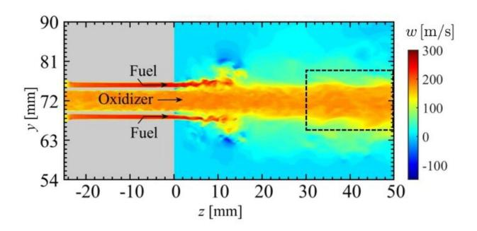
This figure shows that large-scale vortex rings are produced from the injector rim during combustion oscillations. Credit: Satomi Shima, Kosuke Nakamura, Hiroshi Gotoda, Yuya Ohmichi, and Shingo Matsuyama
