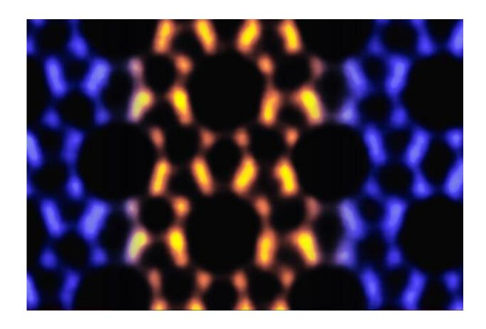
Atomic-scale details from transmission electron microscopy that reveals the porous structure of an MFI nanosheet, with MEL intergrown in it. Credit: Kumar et al., University of Minnesota
