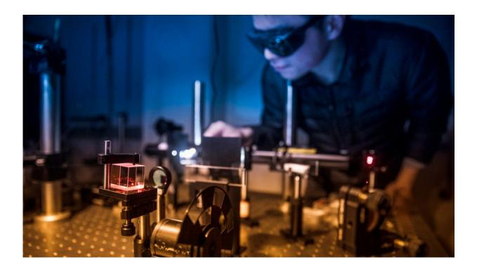
Shengwei Jiang, postdoctoral researcher, aligns an optical setup for magnetooptical Kerr rotation microscopy measurements on atomically thin magnets. Credit: Lindsay France
