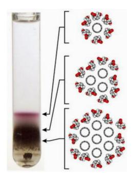
The vial holds a nanotube solution after ultracentriuging has separated it into different layers. The purple layer at the top consists of a highly uniform population of the single-walled semiconductor nanotubes that are the most strongly luminescent. The illustrations at the right show the typical constitutents of each layer. Credit: Tobias Hertel
