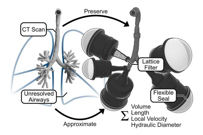
Patient features are preserved in the TIDAL model and distal airways are approximated as 3D printed lattice filters by considering their cumulative regional properties. The TIDAL model is programmed with controllable breathing parameters within an enclosed aerosol delivery space. With the TIDAL system, it is possible to assess spatial aerosol deposition and account for interactions between device, formulation, and patient factors. Credit: *Device* (2024). DOI: 10.1016/j.device.2024.100514
