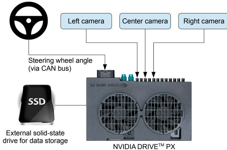
Figure 1: High-level view of the data collection system.
