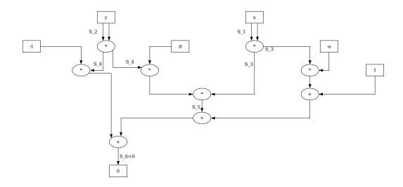
The circuit enforces the two inputs of field type to satisfy the twisted Edwards curve equation and, as we know from example 130, the associated Rank-1 Constraint System is given by:
