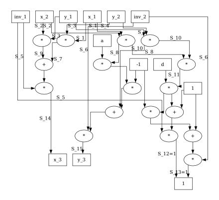
Using the general technique from 6.2.2.4 to derive the associated Rank-1 Constraint System, we get the following result:
