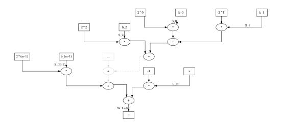
Applying the general transformation rule 6.2.2.4 to compute the associated Rank-1 Constraint Systems, we see that we actually only need a single constraint to enforce some binary representation of any field element. We get
