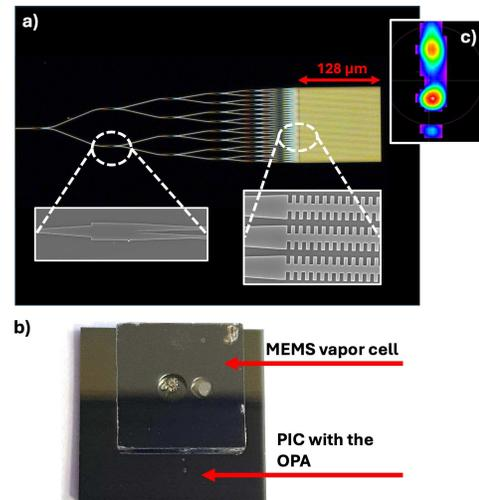
Fig. 1. a) Darkfield microscope image of the optical phased array (OPA) with high magnification SEM images of the MMI coupler and grating antenna as insets. b) Proposed integration method of a MEMS vapour cell with photonic integrated circuits by flip chip bonding. c) Far-field beam profile of the OPA recorded experimentally.
