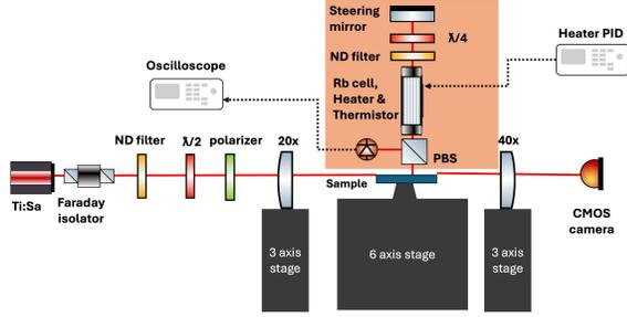
Fig. 2. Measurement set-up for saturated absorption spectroscopy with beam delivered from a photonic integrated circuit including an optical phased array.
