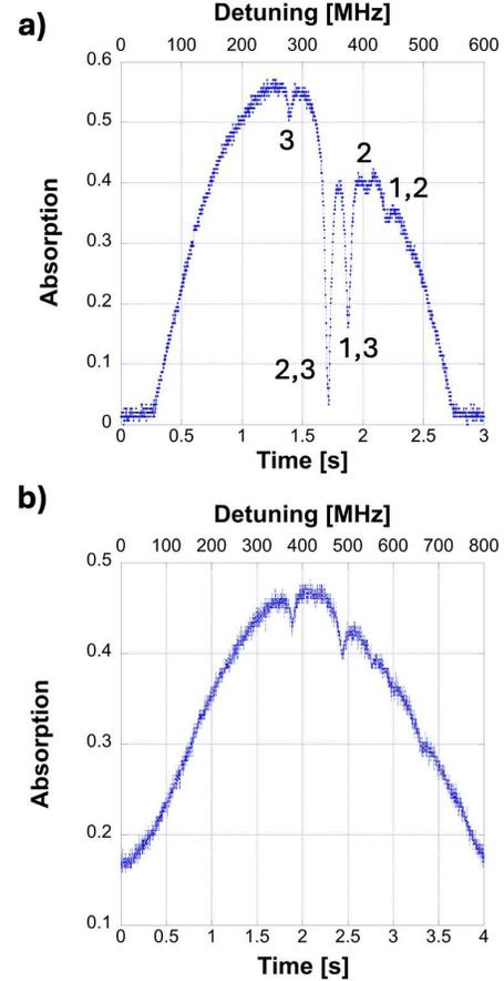
Fig. 3. Normalised absorption of the  $|5S_{1/2}, F_g = 2\rangle \rightarrow |5P_{3/2}\rangle$  transition vs the laser scan time recorded by saturated absorption spectroscopy (SAS) utilising the optical phased array (OPA) for beam delivery. a) SAS utilising a glass vapour cell, numbers labelling hyperfine levels  $F_e$ . b) SAS utilising a MEMS vapour cell.
