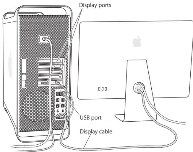
You can connect displays with Mini DisplayPort or Digital Visual Interface (DVI) connectors to the display ports on the back of your Mac Pro. The DVI port is a dual-link port, so you can connect a 30-inch Apple Cinema HD Display.
