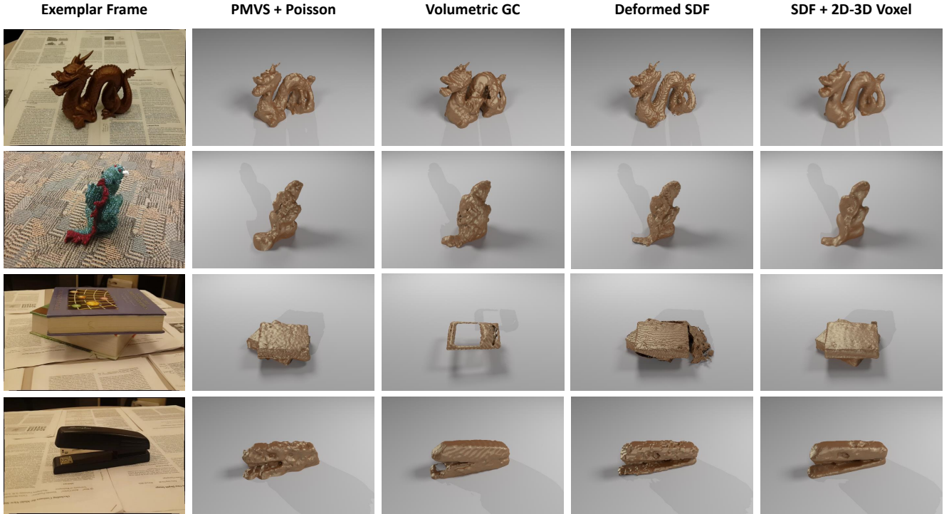
Figure 8: Comparison of reconstructions produced by our system “SDF + 2D-3D Voxel” with other baseline methods on videos in Object-Videos dataset. Our approach incorporates: dense depth maps with an improved cost function and improved signed distance function for fusion; sparse patch-based stereo 3D points (PMVS); and joint 2D-3D segmentation based on color, edge, and depth cues. By using a broad set of techniques, our system avoids many of the errors and artifacts inherent in any individual. Note that our method produces smoother and more detailed reconstructions as compared to the baseline methods while being more robust to errors in PMVS point cloud and depth estimation errors that show their effect in “PMVS + Poisson” and “Deformed SDF”. Also unlike “Volumetric GC”, our approach is less sensitive to the color model, as evident from the books example.
