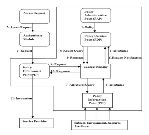
Fig 2: General access control model architecture
