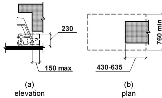
**Figure 6: Toe clearance**
