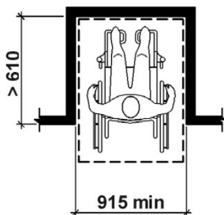
**Figure 4: Manoeuvring Clearance in an Alcove, Forward Approach**
