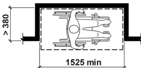
**Figure 5: Manoeuvring Clearance in an Alcove, Parallel Approach**
