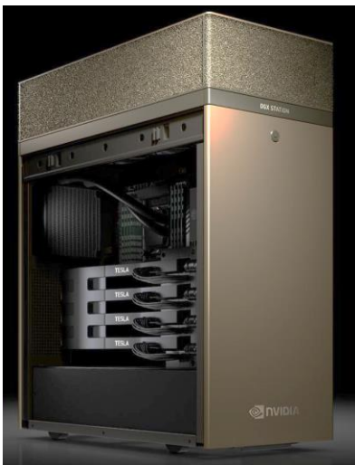
Figure 31. Tesla V100 Powered DGX Station
