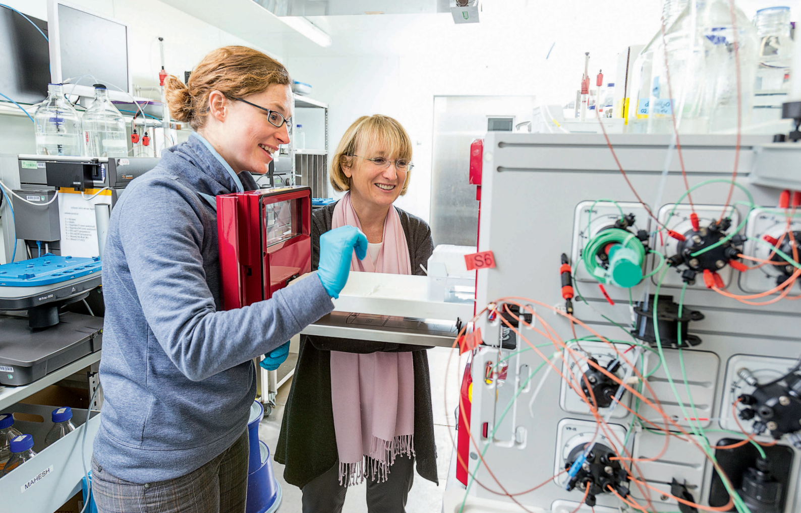
"That's the most exciting part of the day," Elena Conti looks forward to her daily round through the laboratory. Here, she and her colleague Eva Kowalinski (left) are standing in front of a chromatograph, which is used for purifying proteins.
