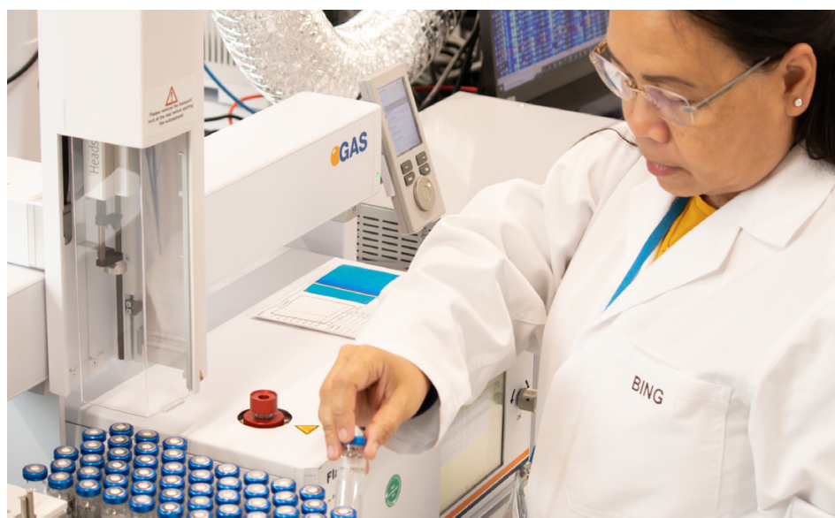
FIG. F.3. Headspace–GC–IMS analysis to detect characteristic fingerprints of food contaminants, performed at the Food Safety and Control Laboratory, Joint FAO/IAEA Centre of Nuclear Techniques in Food and Agriculture, Seibersdorf, Austria. (Photo: IAEA)
