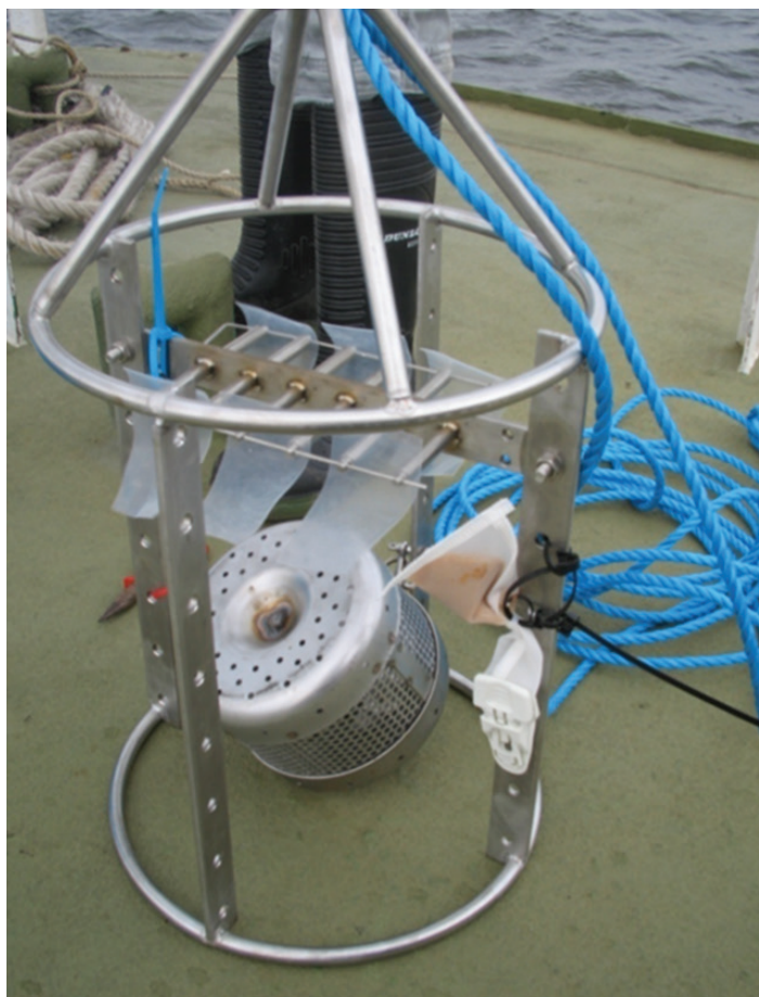
FIG. 1.2. Passive sampling devices ready for deployment at sea. (Photo: Centre for Environment, Fisheries and Aquaculture Science, United Kingdom)
