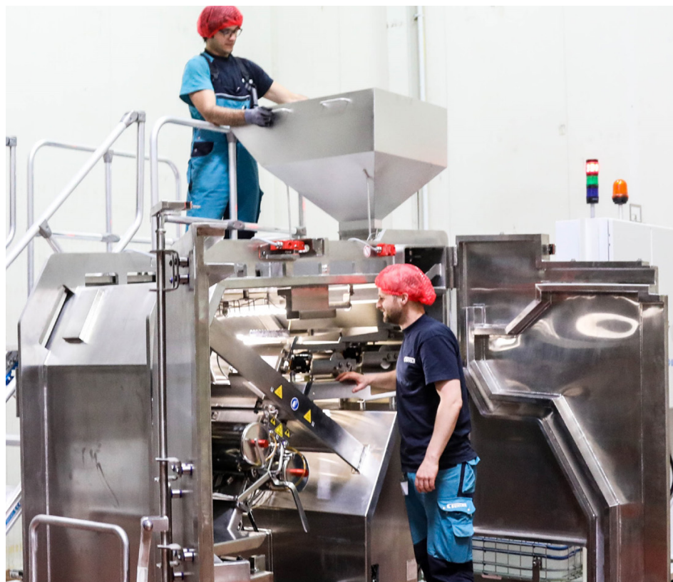
FIG. F.5. Soft electron food processing equipment. The Laatu machine uses two low energy electron lamps (the red handles in the middle of the picture) to process dried ingredients as they fall through a stream of electrons. With a reduced energy consumption of up to 80% less than steam methods, it provides a cost efficient solution for microbial reduction. (Photo: Bühler)
