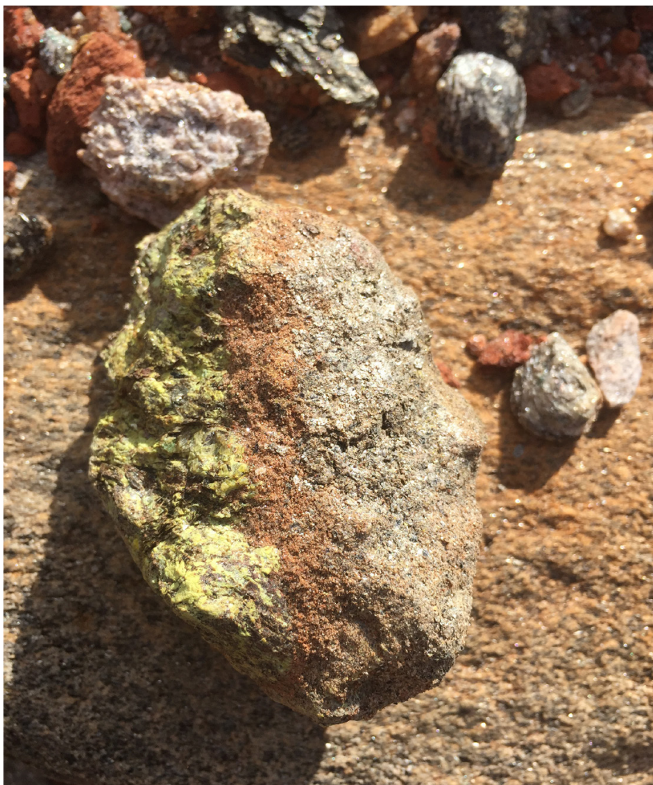
FIG. C.3. Residues from the copper mining industry with the presence of NORM. (Photo: IAEA)
