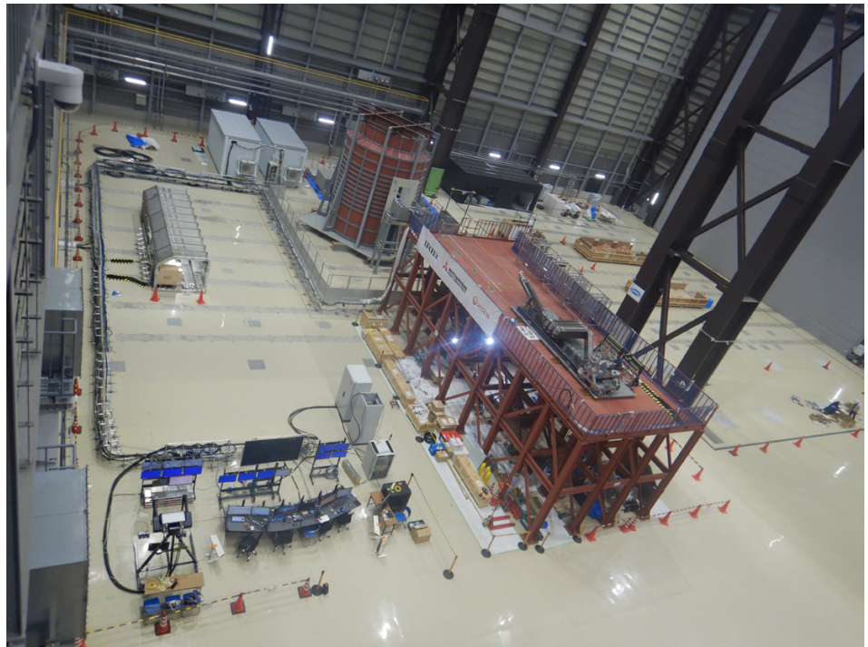
FIG. C.2. Testing hall for robotic arms and manipulators for Fukushima Daiichi NPP. (Photo: Ministry of Economy, Trade and Industry, Japan)
