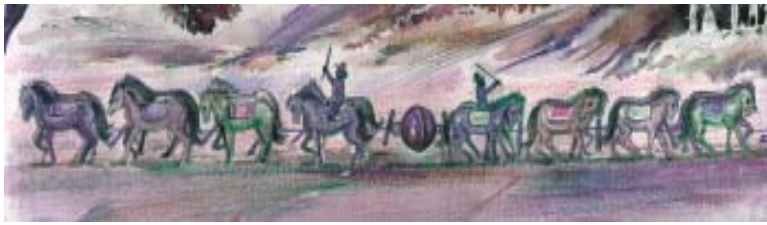
Fig 8.30: Otto von Guericke's experiment to demonstrate the strength of a vacuum, using two 'Magdeburg' hemispheres of brass from which air had been exhausted.
