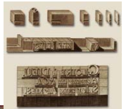
Fig 6.11: Printer's workshop: About 1438 the German metal worker Johannes Gutenberg invented type casting, a method of making movable type from molten metal. This invention was responsible for the rise of humanism by making the classics available to a larger number of people.
