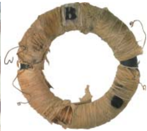
Fig 8.20: Induction coil (Faraday's Ring)
