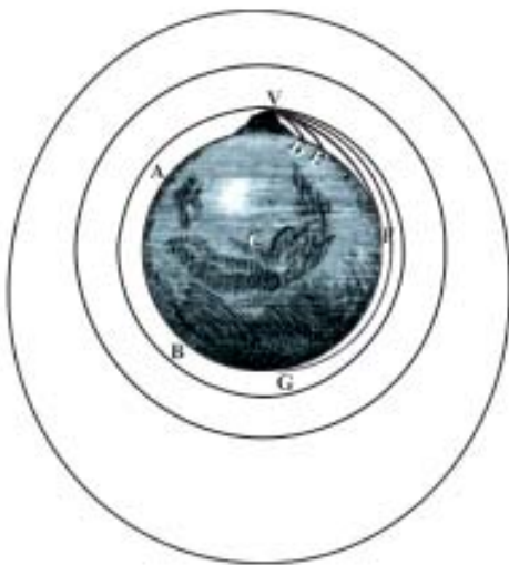
Fig 6.50: Newton's diagram of the flight of a cannon ball: He explained mathematically that the cannon ball, if fired from the top of a mountain with sufficient speed, can be made to orbit the earth.
