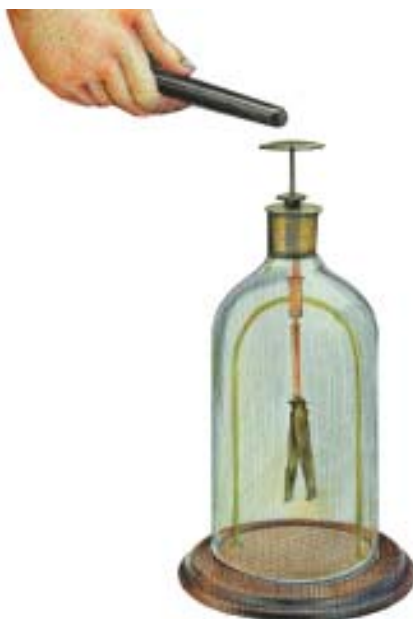
Fig 8.15: Electroscope is an important instrument for detecting electric charge. A positively charged resin rod is held near the top of the electroscopes. The metal rod of the electroscopes gets negatively charged, leaving excess positive charges on the gold leaves, as a result of which the leaves repel each other. The electroscopes were originally invented by William Gilbert who also coined the term electricity in the seventeenth century.
