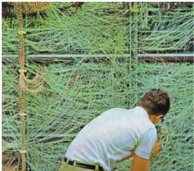
Fig: 19.16: A Univac 490 computer has more than 7,700 printed circuits, requiring 70 miles of wiring to hook up its two million "memory cells". Still the degree of complexity is many times lower than the human brain.
