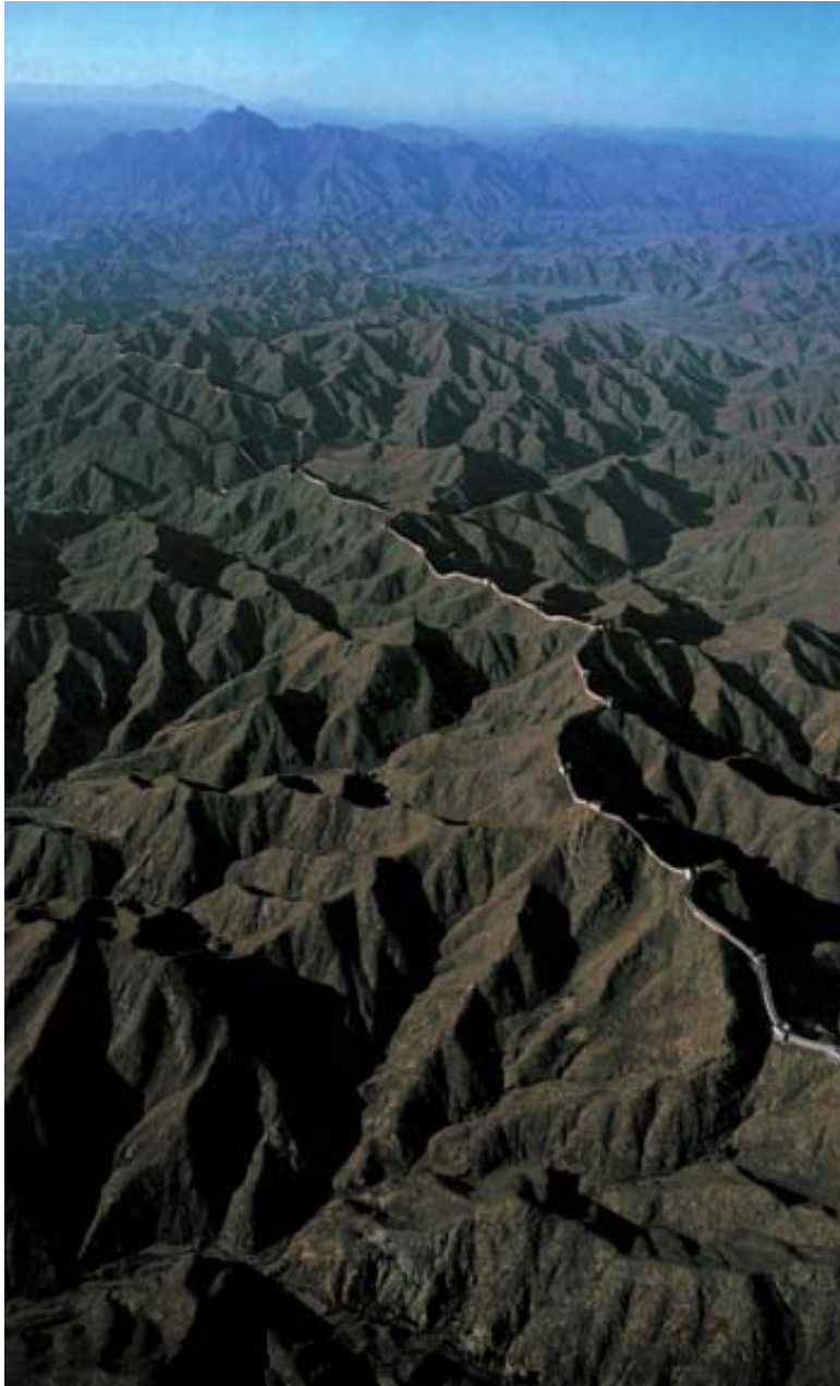
Fig. 4.2: The Great Wall of China , about 2,400 km long and 9 m high at most places, represents one of the largest building projects ever undertaken. It was built during 453-221 BC when a number of small defensive structures were built in the Warring States Period. In 221 BC, Ch'in Shih Huang Ti (Di), the first Emperor of China, connected these, extending the Wall from the Liaoning Province in the east to central Asia in the west. Originally, the structures were built of masonry and earth, with brick faces in some portions. The Wall stands as a testimony to the engineering genius of the Chinese.
