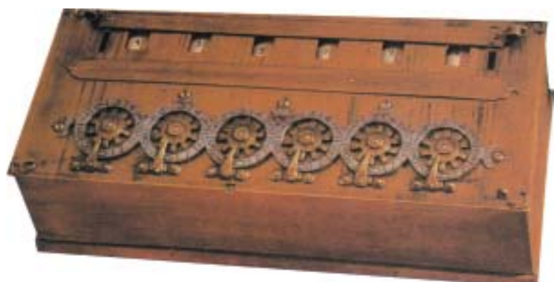
Fig: 19.2: Pascaline , the true ancestor of the modern pocket calculator, was capable of operations with whole numbers. Made by Blaise Pascal in 1662, it worked in the same way as a car odometer.
