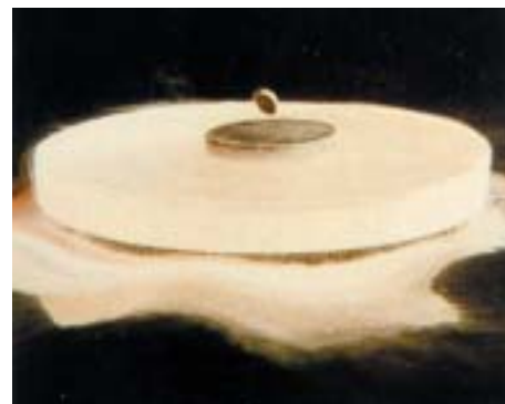
Fig: 17.31: Superconductors , awaiting a technological breakthrough for wide- scale applications. A bar magnet lowered onto a superconducting tin dish creates a magnetic image in the dish, and is therefore repelled by the force between like poles, so that it remains levitated above the dish.
