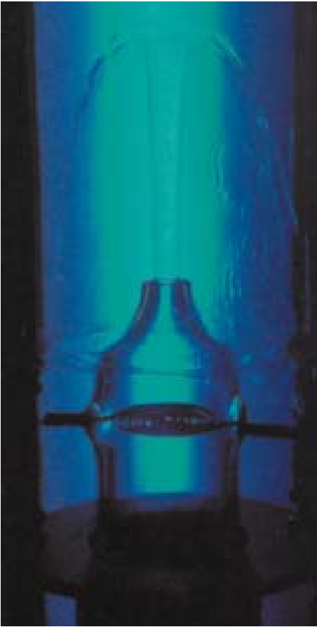
Fig: 16.25: The spectacle of Superfluidity: Below a certain temperature, liquid turns superfluid. It loses its viscosity and acts like a superconductor of heat. A heater in the glass vessel attracts superfluid helium which rushes into the vessel below the heater. The jet of liquid is forced through a small hole at the top producing a fountain.
