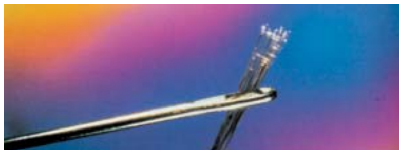
Fig: 17.37: Optical fibres , which have revolutionised communications technology, are so thin that a whole bundle of fibres can pass through the eye of a needle.
