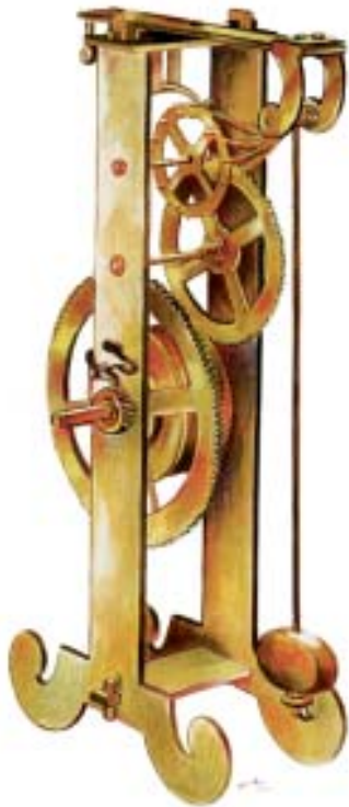
Fig 6.34: Galileo's pendulum clock: Galileo discovered the constancy of the period of the pendulum and devised an idea for adapting a pendulum to control clockwork, although it is not known for certain whether he ever made such an instrument.
