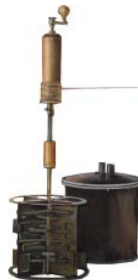
Fig 8.26: Joule experimentally measured the work required to generate heat. Falling weights turned the paddles in a container of water. The water became hot due to friction. Joule measured the rise in temperature of the water and calculated the heat generated.
