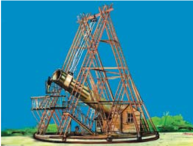
Fig: 11.2: Herschel's telescope: Musician by day and an astronomer by night, Herschel was also a mirror maker. He personally ground and polished the mirrors for his telescopes. The picture shows Herschel's giant reflector which he built in 1780s, with an aperture of 1.2 m and a focal length of not less than 12 m.
