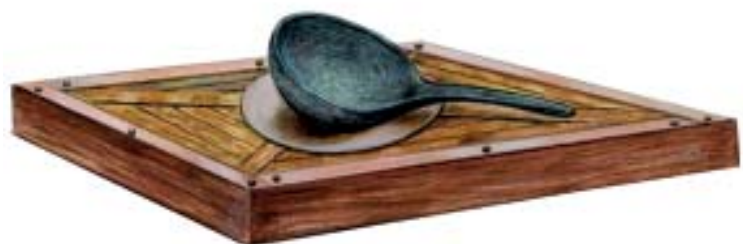
Fig. 4.16: A fortune teller's divining board was the precursor of the magnetic compass. The 'spoon,' made of lodestone, always pointed to the south pole. By the first century AD, the Chinese started designing and using lighter magnetic objects like thin needles mounted on wood. They used the compass first in civil engineering and by the tenth century began using it for navigation.
