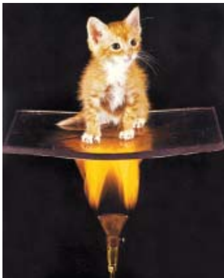
Fig: 17.33: A Cool Kitten: Perched on top of a 2,000 degrees Celsius. flame, this kitten is protected by a slab of silicone called RTV 615, a transparent rubber. Similar silicones, called the space-age substances, are used as heat shields of space vehicles and can withstand the temperatures of 8,000 degrees Celsius.
