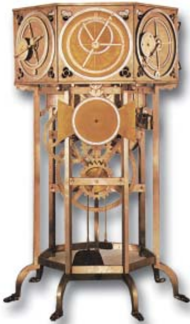
Fig 6.1: A weight-driven astronomical clock constructed by Giovanni de Dondi: The upper dials trace, from the left, movements of Mars, the Sun and Venus; the lower dial is a 24-hour clock. The early mechanical clocks were regulated by a verge and foliot escapement. It was driven by a weight that hung down below the clock as shown at the bottom of this panel.
