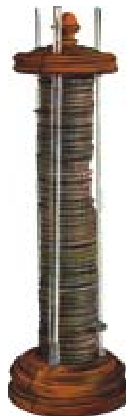
Fig 8.18: Alessandro Volta (1745-1827) and the Pile: Volta used three components to make a cell: zinc, cardboard/leather (soaked in a salt solution or vinegar) and copper. He piled these cells and produced the first chemical battery in 1800.
