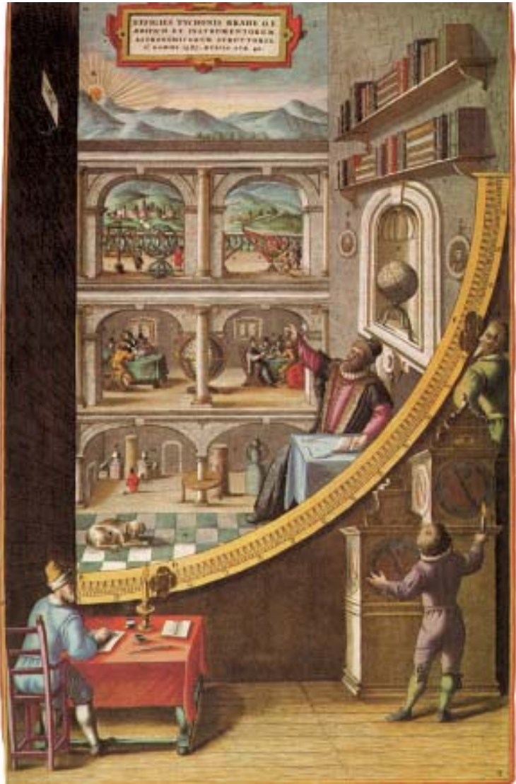
Fig 6.26: Tycho's Mural Quadrant, a huge brass arc of 6 feet radius was built in his observatory in 1576
