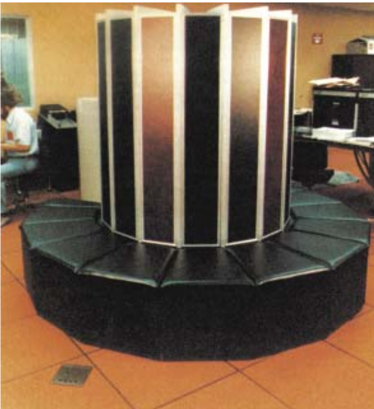
Fig: 19.23: Cray-1 Super Computer, made in 1976 was capable of 700 million operations a second.
