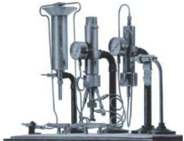
Fig: 17.24: Haber-Bosch process heralded a new era in the chemical industry. Ammonia was synthesised from air in the laboratory by Nobel Laureate (1918) Fritz Haber and in a high pressure reactor by Nobel Laureate (1931) Carl Bosch.
