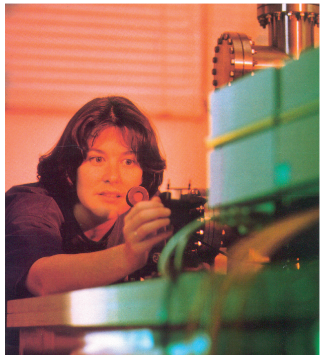
Figure 21: An illustration of laboratory astrophysics: aligning the optics for a laser spectroscopic measurement.
