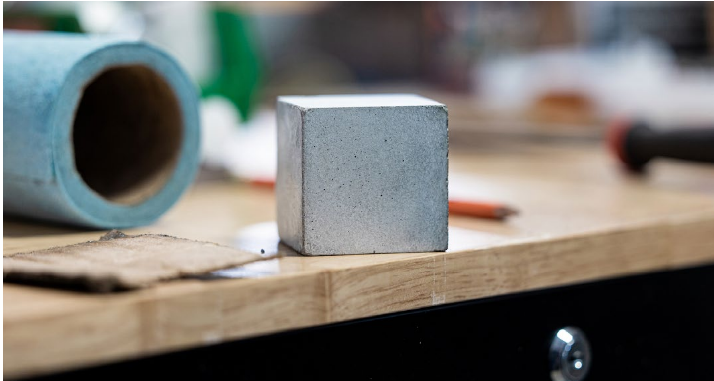
► Brimstone made this cube of concrete using cement from carbon-free calcium silicate rocks.
