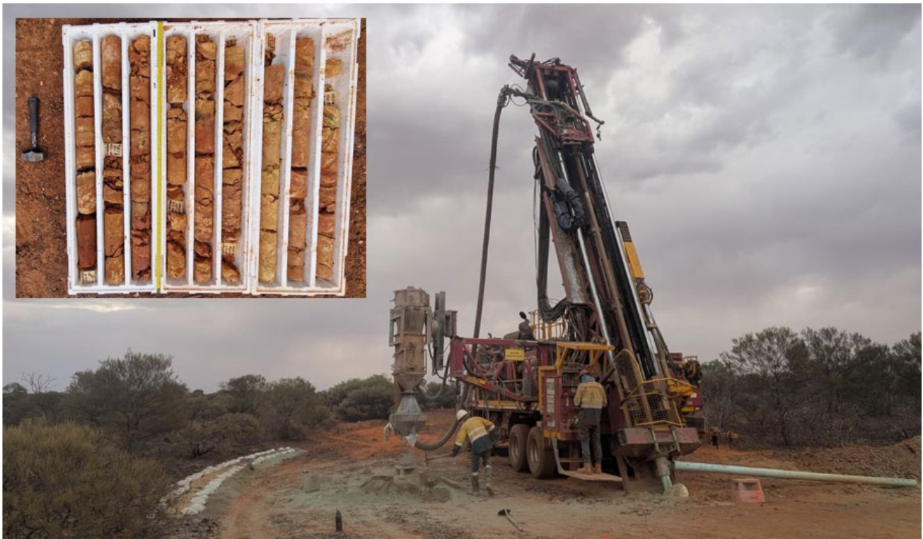
Figure 8 – Diamon rig drilling wide diametre core for heap leach amenability and gold recovery testwork on near surface gold bearing oxide and transition material. The inset image shows the oxide core from first drill hole.
