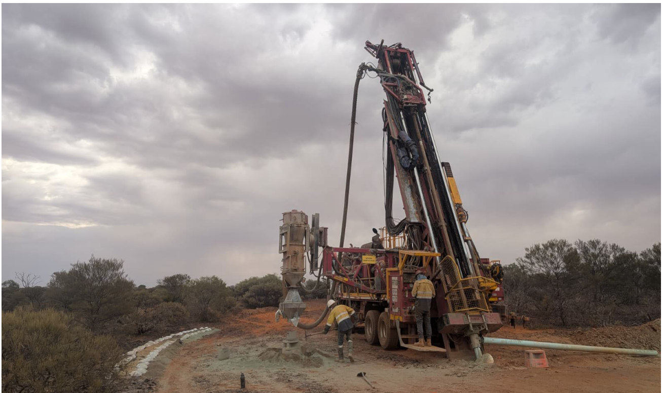
Figure 2 – RC drilling of first hole at the Shiraz gold prospect designed to test a high-grade diamond intersection (6m@ 4.2g/t gold) located approximately 215 vertical metres below a near-surface gold saprolite zone.
