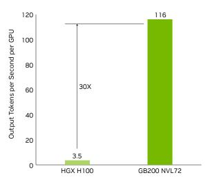
Projected performance, subject to change. LLM inference and energy efficiency: token-to-token latency (TTL) = 50 milliseconds (ms) real time, first token latency (FTL) = 5s, 32,768 input/1,024 output, NVIDIA HGX™ H100 scaled over InfiniBand (IB) versus GB200 NVL72.
