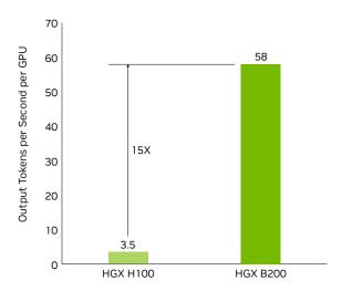
Projected performance, subject to change. Token-to-token latency (TTL) = 50ms real time, first token latency (FTL) = 5s, input sequence length = 32,768, output sequence length = 1,028, 8x eight-way HGX H100 GPUs aircooled versus 1x eight-way HGX B200 air-cooled, per GPU performance comparison
