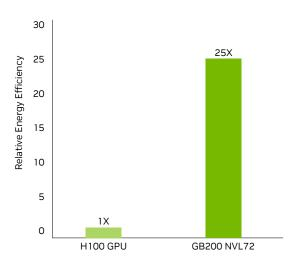
Projected performance, subject to change. Energy savings for 65 racks eight-way HGX H100 air-cooled versus one rack GB200 NLV72 liquid-cooled with equivalent performance on GPT MoE 1.8T real-time inference throughput.
