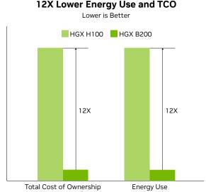
Projected performance, subject to change. Token-to-token latency (TTL) = 50ms real time, first token latency (FTL) = 5s, input sequence length = 32,768, output sequence length = 1,028, 8x eight-way HGX H100 GPUs air-cooled versus 1x eight-way HGX B200 air-cooled, per GPU performance comparison. TCO and energy savings for 100 racks eight-way HGX H100 air-cooled versus 8 racks eight-way HGX B200 air-cooled with equivalent performance.
