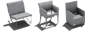
Figure 3: Undesirable artifacts produced by naïve DDPM due to the sensitivity of marching tetrahedra to SDF noises. Better viewed by zooming in.
