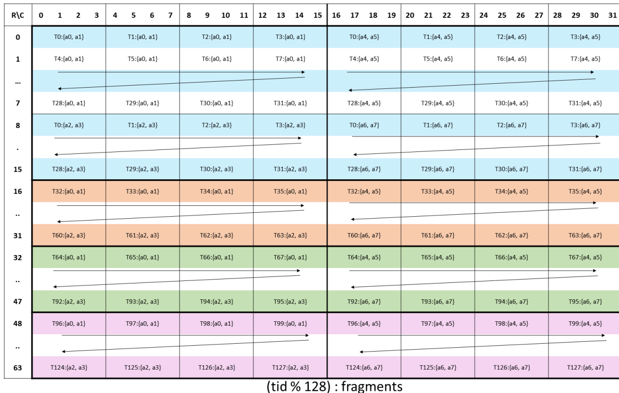
Figure 174: Sparse WGMMA .m64nNk32 fragment layout for matrix A with .f16/.bf16 type.
