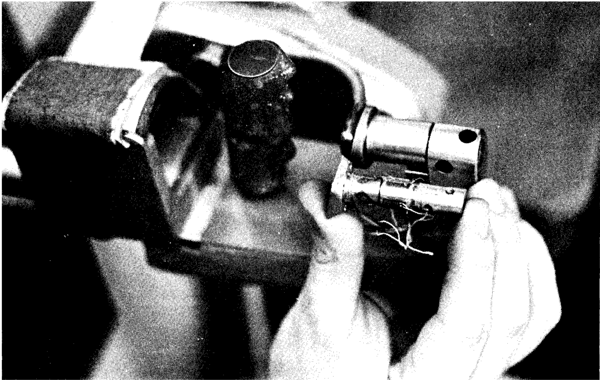
Figure 6 Gage Position for Wrist Transducer Used to Measure pronation/Supination, Flexion/Extension, and Adduction/Abduction. (See also Figure 10)
