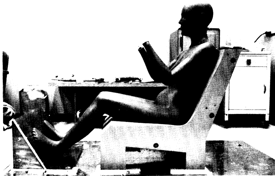
FIGURE 4-7. Sculpting the small female model using HBX-2 clay.
