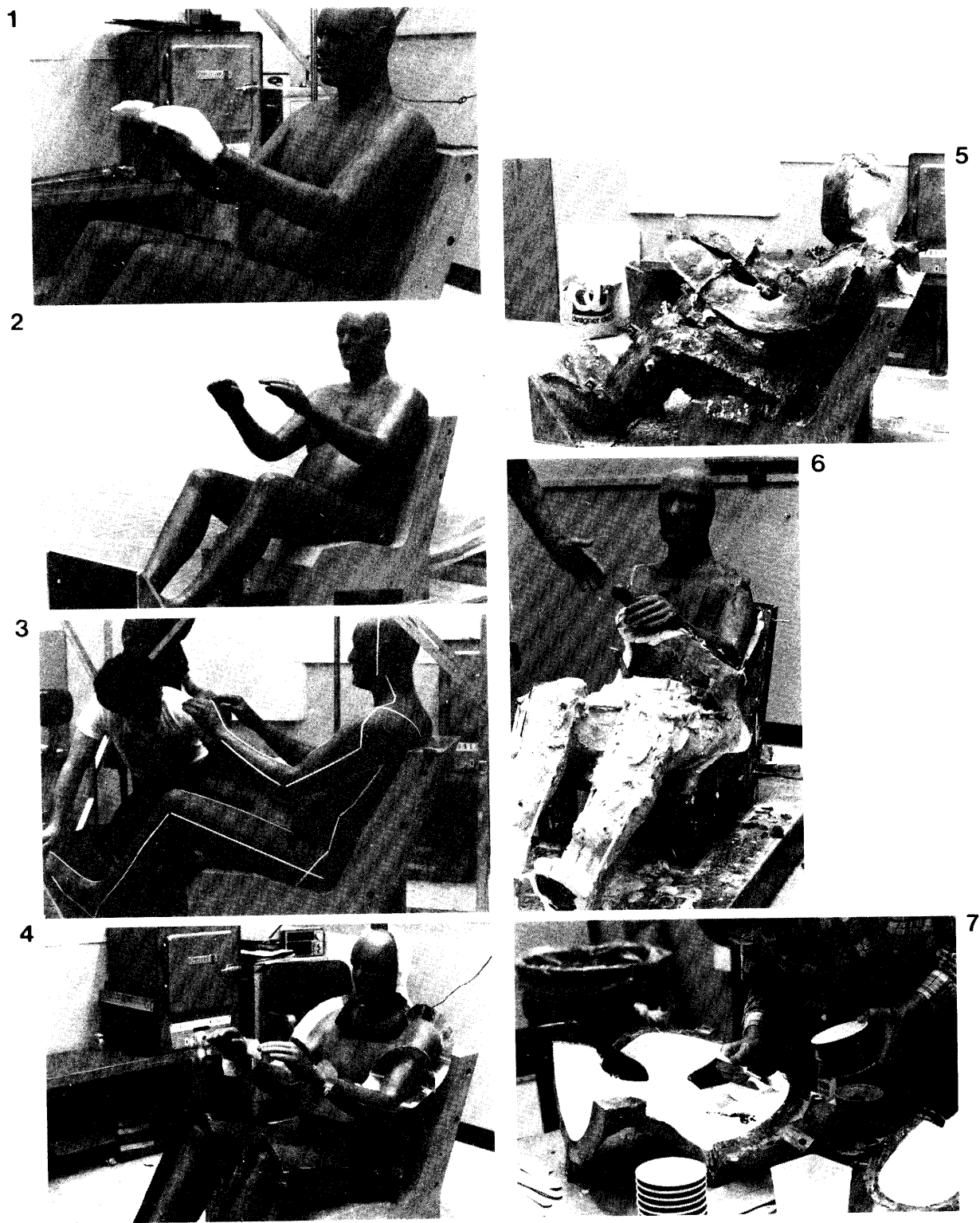
FIGURE J-5. Completing the large male clay model and making the plaster/hemp mold.
