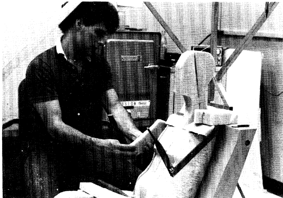
FIGURE 4-4. Attaching styrofoam to welded steel armature.
