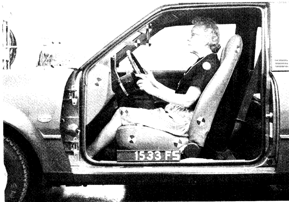
FIGURE 3-4. Small female subject sitting in Ford Escort showing a significant difference between "normal" (above) and "standardized" (below) seated postures.
