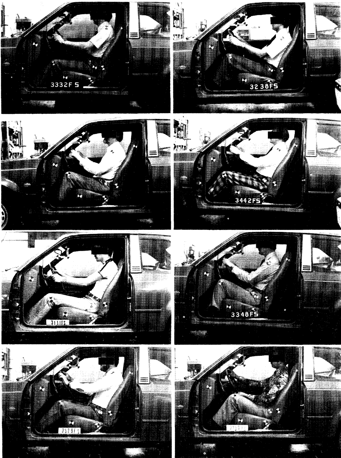
FIGURE A-4. Examples of the "standardized normal driving posture" for eight mid-sized males in the Ford Escort.
