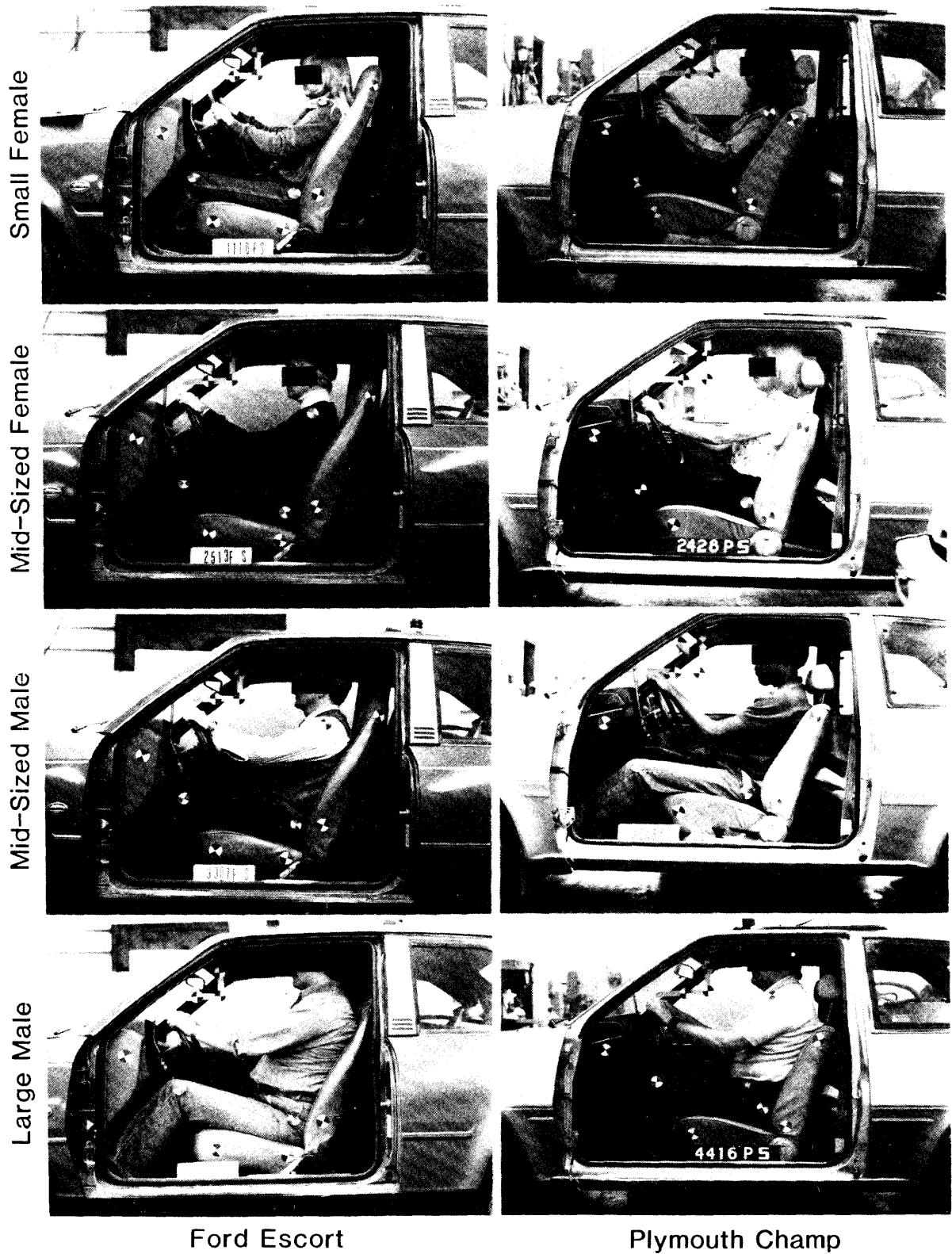
FIGURE A-1. Examples of the "standardized normal driving posture" for the four subject groups in the Ford Escort and Plymouth Champ.
